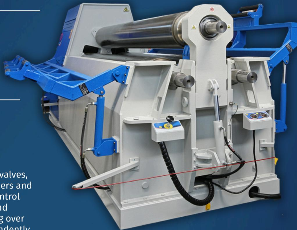
Two proportional solenoid valves, two digital readout transducers and a dedicated electronic control guarantee precision and repeatability of positioning over time for each roller, independently of the temperature and any mechanical wear, always guaranteeing maximum precision.
